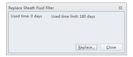
Select **Replace**. A pop-up window appears to reset the maintenance date as the current date that the maintenance was performed.
