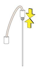
**12** [Without Sample Injection Mode Control Kit]: Connect the sample PEEK tubing to the sample peristaltic pump tubing.
