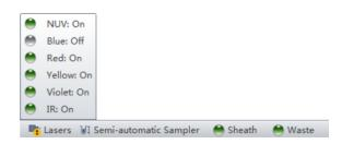
**NOTE** Lasers can only be enabled and disabled when the system is in standby mode.
